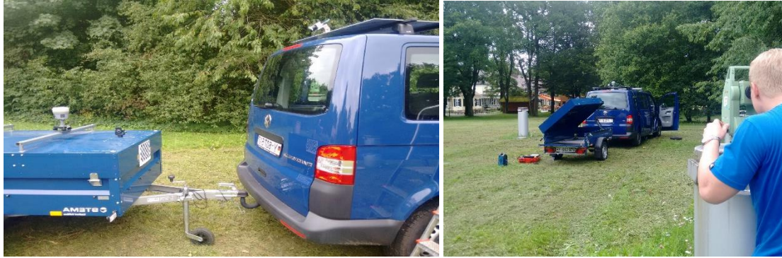
Figure 8: (Left) Hardware setup for the measurement (right) theodolite setup to obtain reference orientation
