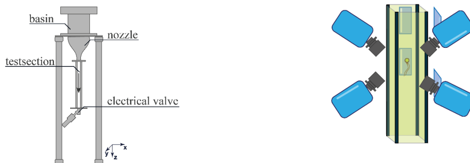
Figure 2 Schematic diagram of the countercurrent channel (left). The flow velocity is regulated by an electric valve at the end of the measuring section. In order to generate a continuous flow, the fluid is pumped back into the water basin. The turbulence generators are located between the measuring section and the nozzle. Schematic representation of the camera setup (right) with controlled background lighting. White LEDs are used as backlight for better contrast in the shadows.
