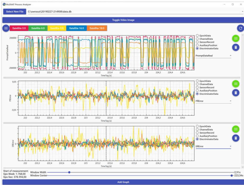
Fig. 3: Screenshot of MuSNAT-Analyzer (alpha-version) with correlator, Phase Lock Loop (PLL) discriminator and Delay Lock Loop (DLL) discriminator values for several GPS C/A signals
