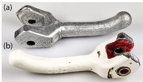
Figure 7. Spare directly printed from scan (a) compared to the original part (b).
