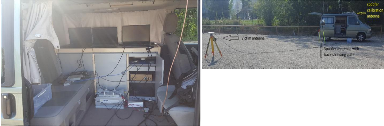
Figure 4: On the left the inner of the measurement bus with the three receivers on the back seat (in front U-Blox M8T, in the middle the IFEN Sx3 and in the background the Septentrio PolaRx5TR). In the drawers the LOKI-spoofing. On the bottom the power supply battery with a power converter. On the right the victim antenna (front) and spoofer antenna (back).
