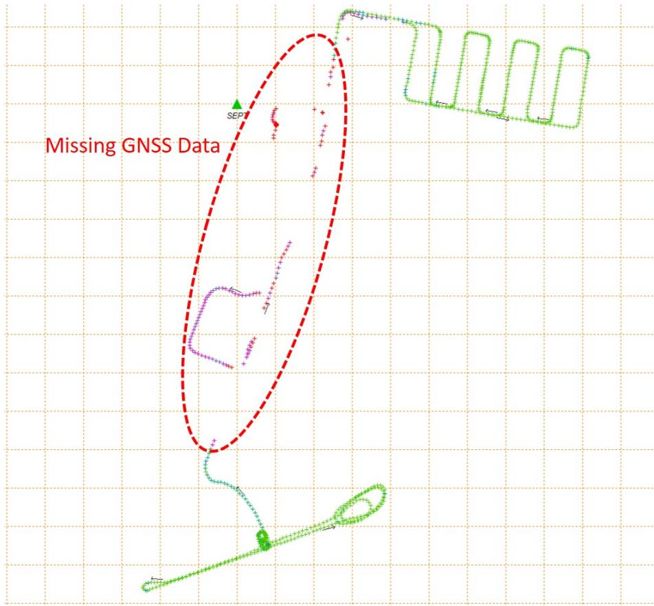
**Figure 7:** GNSS Only Trajectory with Re-transmission Setup
