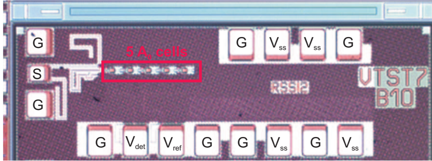
Figure 2.9: Micro photograph of the logarithmic amplifier in B11HFC.
