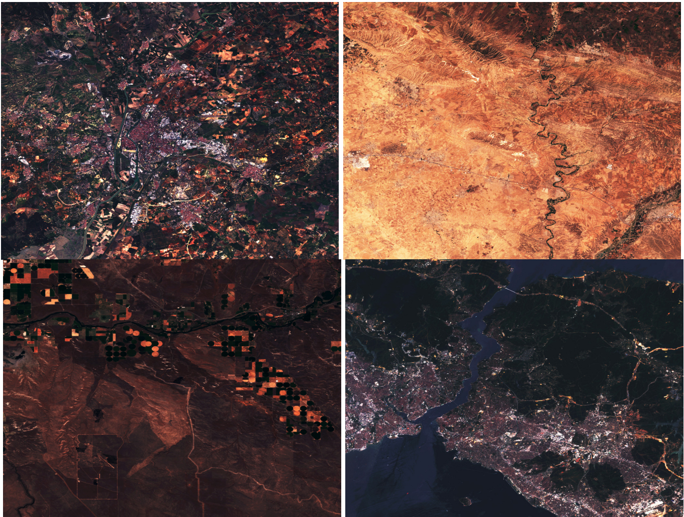
Fig. 6. Four different regions contained in SEN12MS-CR-TS, highlighting the diversity of sampled landcovers. The depicted S2 observations (RGB channels) are cloud-free samples of their respective time series. The average ROI covers about 40 \times 40 \text{ km}^2 and is split into over 700 patch samples, with each patch of size 256 \times 256 \text{ px}^2 .
