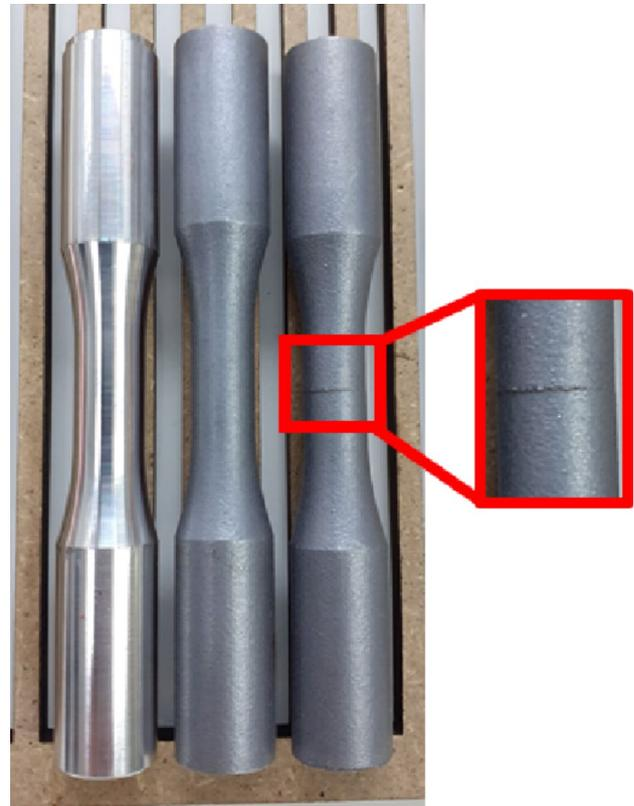
**Fig. 12** Types of fatigue specimens: machined fatigue specimens (left), as-built specimens without interruption (center) and as-built specimens with a 10 h interruption (right)
