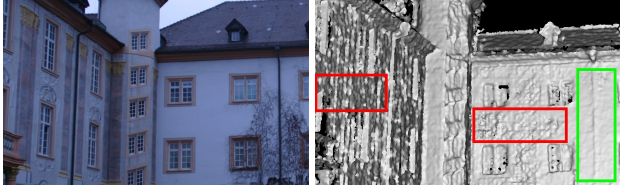
Figure 3. Varying disparity quality. Left: Zoomed region of an input image of the Ettlingen30 sequence [25]. Right: Surface orientation of the disparity map computed by SGM visualized using a linear coding from 0^\circ (light) to 90^\circ (dark). The surface orientation gives a good impression of the reconstruction quality. Accuracy is lower in slanted and untextured regions (left and right red box), and higher in textured fronto-parallel regions (green box).
