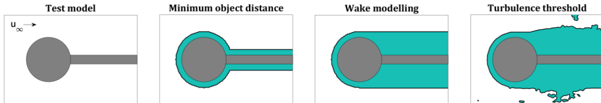
Figure 3: Definition of interface between rotational (green) and irrotational flow domain (white).
