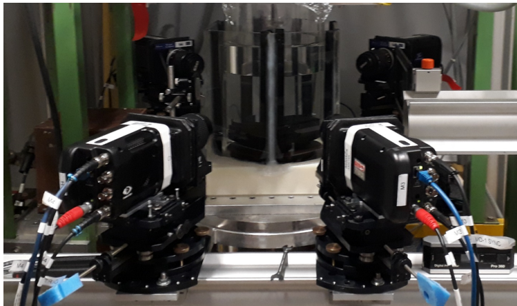
(c) Camera setup around the tank
