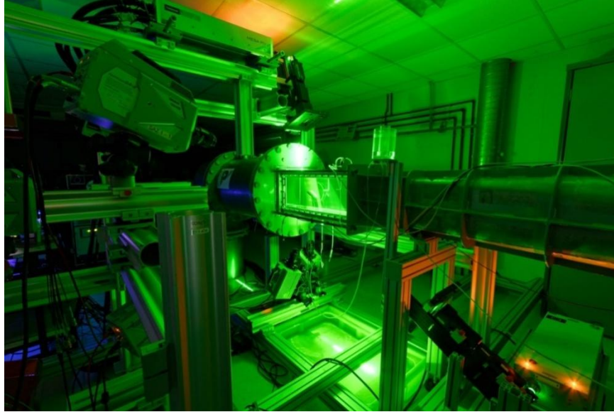
Figure 2: Experimental device of the test section with the two lasers and the six cameras.
