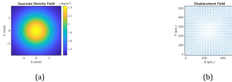
Figure 2. (a) 2D slice of the density field used to render the synthetic BOS images, and (b) the corresponding displacement field.
