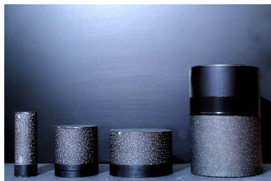
Figure 6: View of the 4 calibrated cylinders with speckled dots
