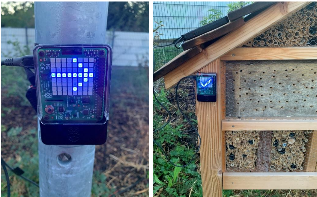
Fig. 7: Micro-Information Radiators deployed at the Senior-Scooter-Park of SHMG that are part of the SUO network which communicates with the activity support service
