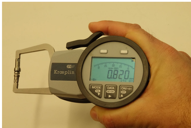
Figure 3.9: Electronic measuring Gauge C1X018 (Kröplin GmbH, Schlüchtern, Germany) as used for ear thickness determination.
