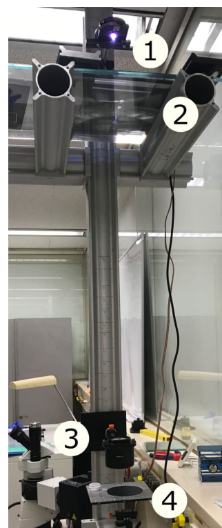
Fig. 2 ①: Light source ②: condenser and photomask ③: objective lens ④: imaging plane and substrate
