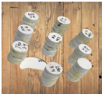
Step 4: 9 LOM-manufactured discs
