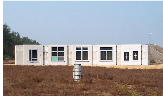
Fig. 10 Typical test setup for a full-scale free field test with several test objects (source: company Bollrath)
