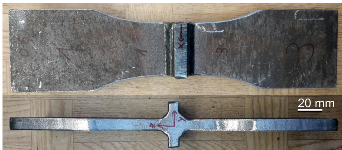
FIGURE 1 Cruciform joint: sheets 15 mm thick, metal active gas welding PA 135, K-seam with full penetration welding, samples provided by industry partners.
