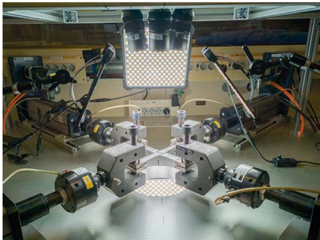
Fig. 7. Biaxial testing machine and DIC system.
