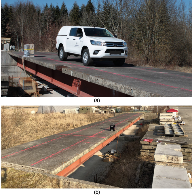
Fig. 6 a) Vehicle for load tests and b) the test bridge as seen from the abutment West
