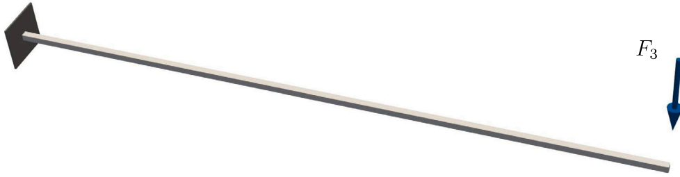
Fig. 2. Cantilever beam under impulsive load: geometry and applied forces.
